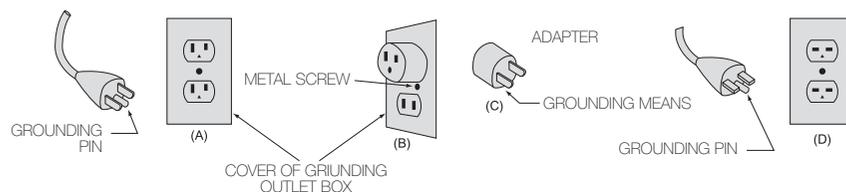
8. USE PROPER EXTENSION CORD. Make sure your extension cord is in good condition. When using an extension cord, be sure to use one heavy enough to carry the current your product will draw. An undersized cord will cause a drop in line voltage resulting in loss of power and overheating. Table (below) shows the correct size to use depending on cord length and nameplate ampere rating. If in doubt, use the next heavier gauge. The smaller the gauge number, the heavier the cord.
