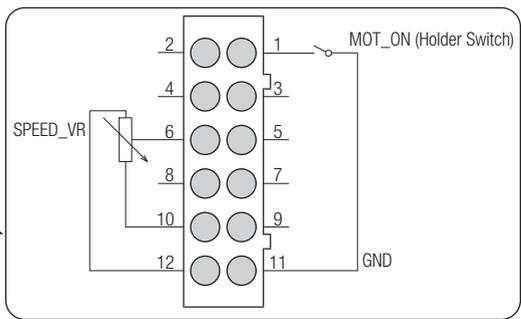
The transistor (open collector output type) can also be used instead of the switch and potentiometer. When your chair unit is controlled by micromotor based, the motor speed control can also be adjusted by installing a DA converter, instead of potentiometer.
