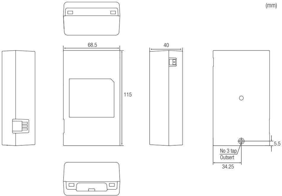
For Installing the NLX BF Control Board with your chair unit, use a screw, or use Velcro (Magic Fastener (1) and (2)).
