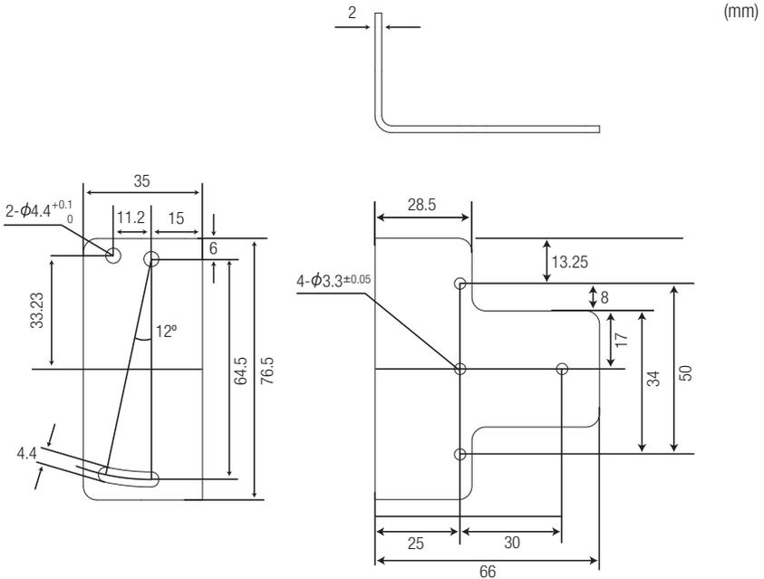
When installing the bracket with your chair unit, use the M3 screws. These screws are not included due to variation of the chair instruments.
